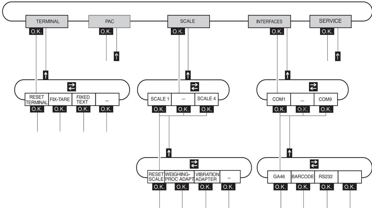
**TERMINAL** For system settings, such as entering the date and time or loading permanent texts, see section 5.3.
